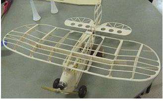
Top left is Reeder Jones' Goldberg Ex-Treme 330 ARF. Reeder put a .46 FX engine in this 3-D machine. Looks very hot! Above left is Don Johnson's latest Lazy Bee in bare bones. It has a PJS 1000 installed and will probably fly with a 9X4.5 APC prop and 10 KAN 1050 NiMH cells. It should weigh in at less than 28 ounces and develop about 100 watts per pound. Not quite a 1:1 power to weight ratio but close.
