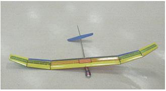
Top right can be nothing other than a Larry Gliser fan fold foam building construction material project. This is a Tim Hart design 3D plane and sports a JPS 1000 motor, 12X6 prop and Lithium-Polymer battery. Larry says it is a very slow flyer. The plans are a free download if you're interested. Above right is Jim Halbert's newest project. A full house Wind Dance competition powered glider. Think it has a geared Mega motor and will fly with 9 to 10 NiMH cells
