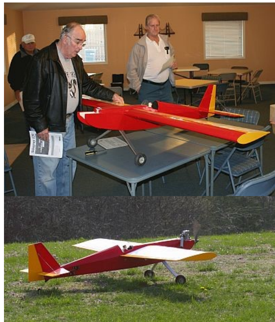
Above is Bud Austin's new Balsa U.S.A. Stingray. A real balsa and ply kit. He hung a big 150 4-stroke engine on the front and it will go straight up. Nice job, Bud.
