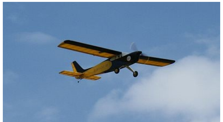
Don Johnson's new stick and tissue Pussycat. Don has built five Pussycats, two with 61.5 wingspans and then three of the 80% version with 50.4" wingspan. They have all flown very well.
