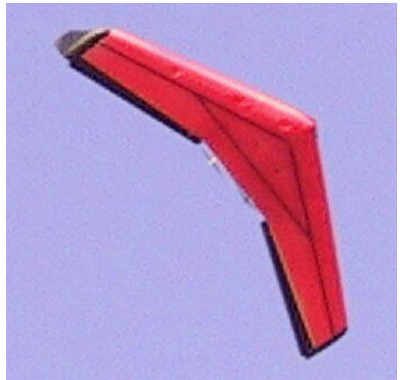
Above is Ray Dixon's VIPER twin Speed 400 electric on a pass over the field. Except for ailerons and canopy cover, this is an all molded foam plane - including the wing tips. Note the dents in the foam on the bottom from hard landings. This is a good flying plane and will do loops and rolls with ease - fast too.
