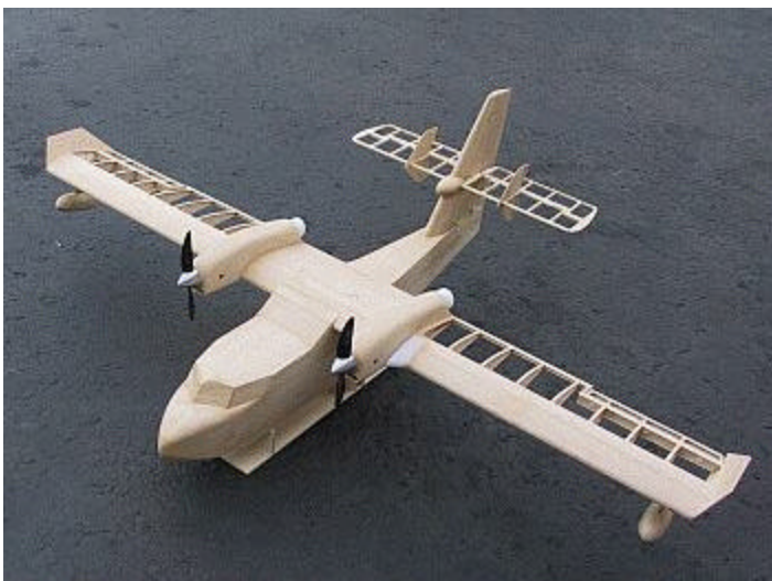
Left is Don Johnson's CANADAIR CL-415 Fire Fighter. Built from magazine plans it has a wingspan of almost 64 inches, twin Speed 400 7.2V motors and 10 1250 mAH nicads and should weigh about 4.5 pounds when ready to fly. It is being finished in Silkspan and Dope. Painting will have to wait until it warms up some so the garage can be ventilated.
